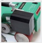
More contact force: Having the centre of gravity directly above the contact roller creates even more pressure, thus allowing a constant weld quality for all types of membrane.
