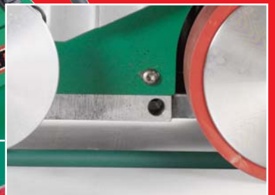
Air partition for homogenous welding seam
