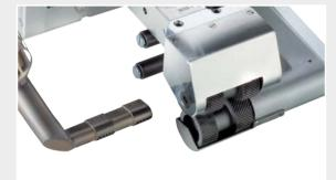
The tightness is the most important criterion when evaluating the weld quality. To guarantee the greatest possible safety here, a test channel is installed for each overlap weld. This is realised with the pressure roller on the TWINNY S which was specially designed for this purpose. This ensures two parallel weld seams of 15 mm each. The test channel that results between these seams is 20 mm wide. The watertightness can be reliably monitored via compressed air using this channel.
