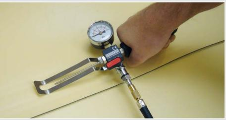
Easy and precise non-destructive seam testing on the construction site
