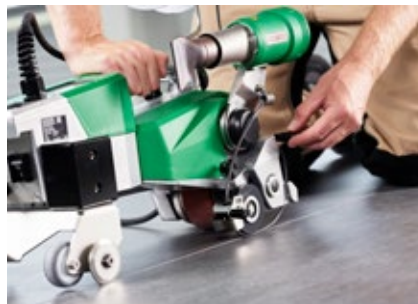
Welding rod pressure roller can be raised and locked
