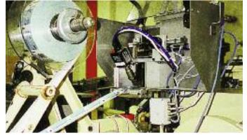
Air heater and blower for drying labels. Fast drying allows for high throughput speeds.
