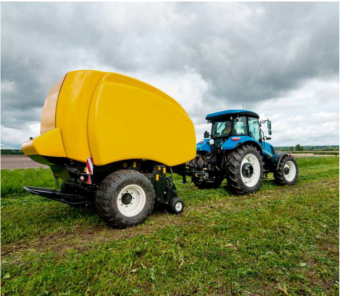
Application example agricultural machinery: Thermoformed tractor cladding such as hood, fenders, cab interior and trailer
