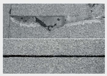
Detailed comparison of two weld seams with open flame (top) and BITUMAT B2 (bottom).
