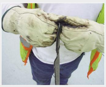
The peel test demonstrates that the weld seam strength is significantly better with the BITUMAT B2 than with a naked flame.
