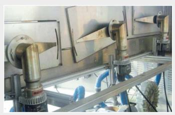
Alignment of Leister wide slot nozzles to shrinking material.
