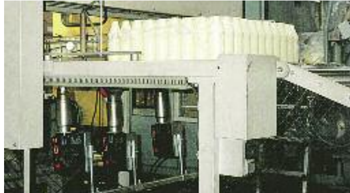
HOTWIND hot air blowers shrink the film on bulky packages.
