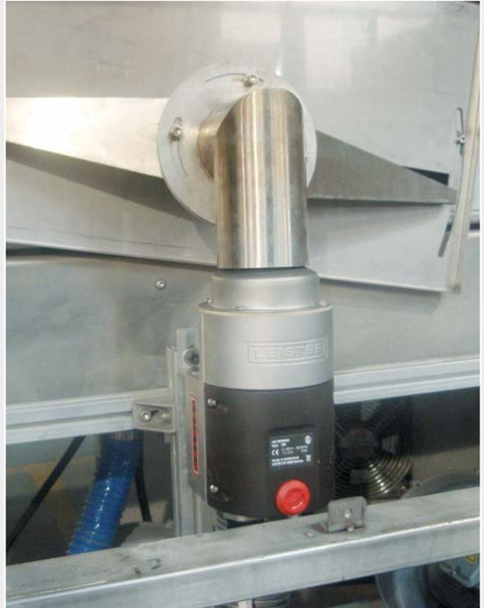
***New air heater LHS PREMIUM 60S with wide slot nozzle installed in a prototype system.***
