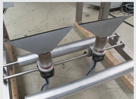
2 of 4 LHS 61L SYSTEM air heaters with their wide slot nozzles
